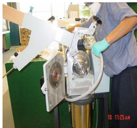
Cleaning of milling device after each operation.
