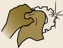
**Use solution with correct inhibitors and dry parts immediately after cleaning to prevent rusting**
