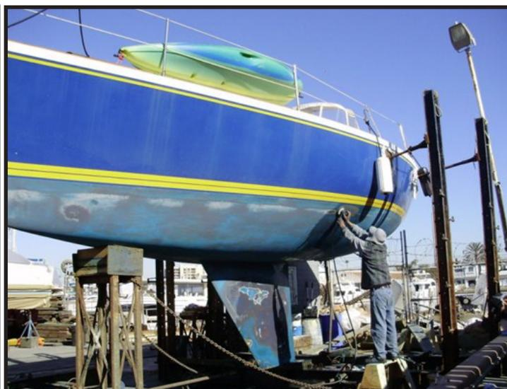
A primer is applied to these spots and then copper topcoat is applied over the prepared hull surface. In some cases, the hull paint is stripped from the boat, often using hand sanding methods. The hand sanding dust from surface preparation or stripping is the second waste stream that contains copper. Some boatyards are starting to use abrasive blasting media to strip boats and the spent media is the third waste stream that contains copper.
