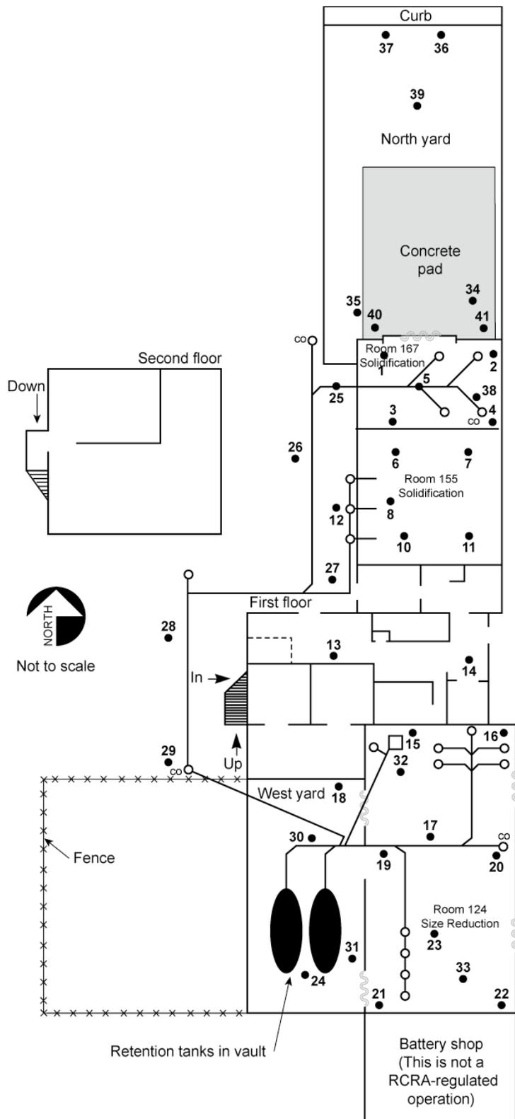
**Figure A-2. Sample borehole locations at the B-419 Facility**
