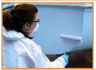
Painting: Both interiors and exteriors of vessels are painted to improve appearance, and to provide corrosion protection. Paint can be sprayed, rolled or brushed onto vessel surfaces. Most top side and interior paints are not as toxic as antifouling bottom paints. The bottom paints, also known as hull paints; generally contain heavy metals such as copper and zinc. On rare occasions, tributyl tin from historic coatings may still remain on hull surfaces.
